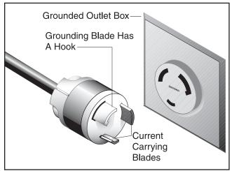
Figure 4. NEMA L6-30 plug and receptacle.
